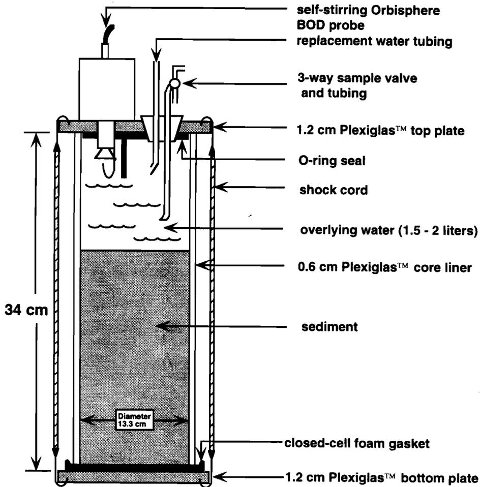
**Figure 3-2. Schematic Diagram of the Incubation Chamber**
